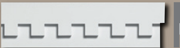
MD 1289 • 1 1/2" Projection • 7" Height • 12'0" Length • 3 1/16" Repeat • 1 1/2" Dentil
