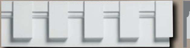
MD 1243 • 1 3/16" Projection • 7" Height • 12'0" Length • 5 3/8" Repeat • 2 7/8" x 5 5/8" Dentil
