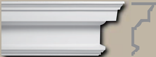
MD 1192 • 9" Projection • 19 1/8" Height • 12'0" Length • Assembled Moulding
